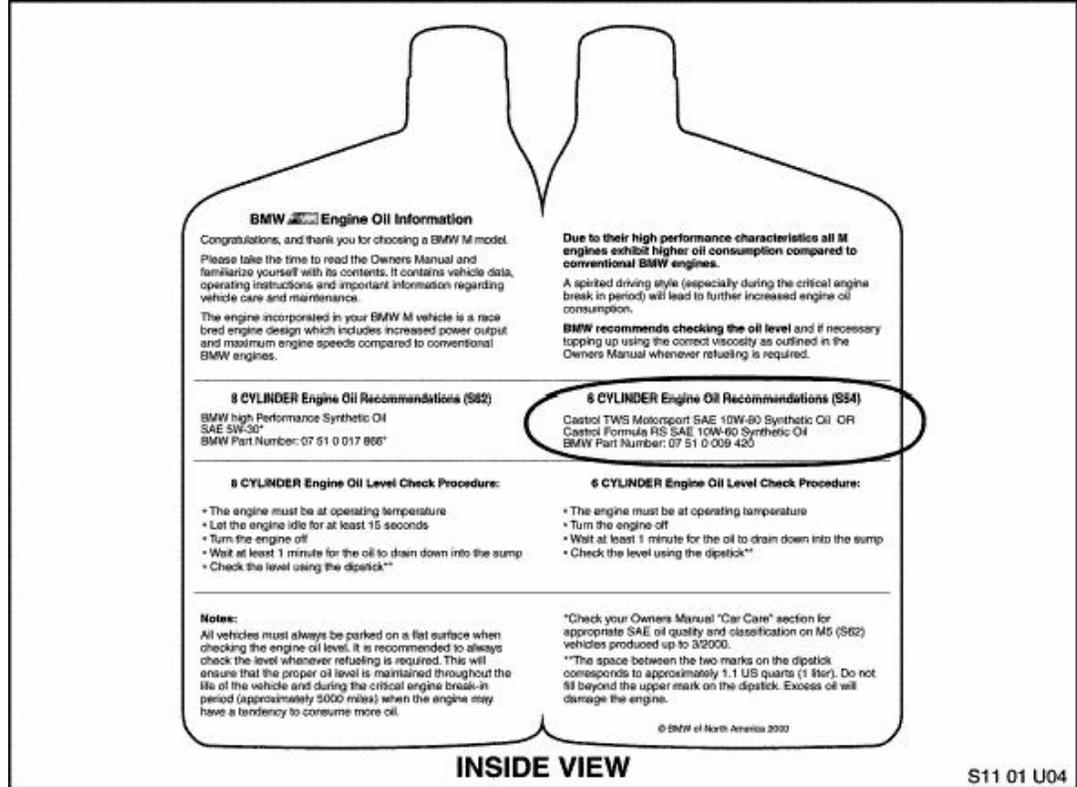
Note: All S54 Engines now use Castrol Formula RS SAE 10W-60 or Castrol TWS Motorsport SAE 10W-60 Synthetic Oil.
