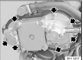
Release screws on VANOS adjustment unit.
