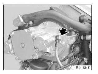
Remove oil line from VANOS adjustment unit.
