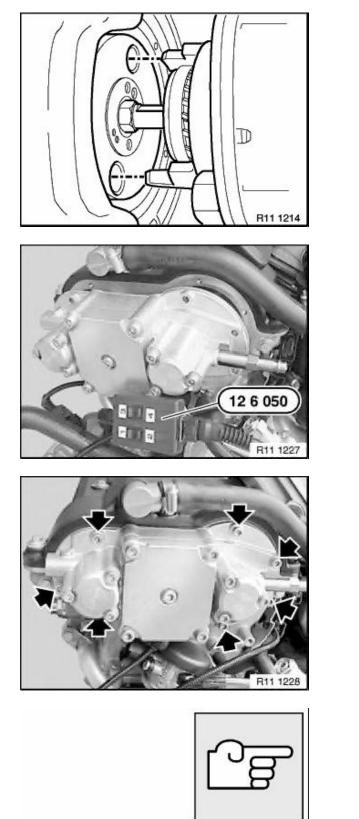
Align radial piston pump to driver on spline hub.
