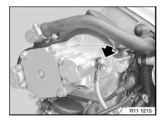
Remove special tool 11 7 130 from VANOS adjustment unit. Fit oil line to VANOS adjustment unit. Tightening torque, refer to 11 36 9AZ. Assemble engine.
